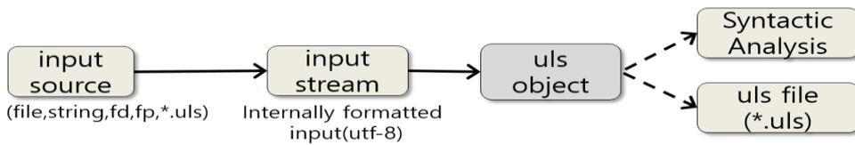
The analyzer object is created by reading the lexical configuration file whose suffix is '.ulc'. The ulc-file is a utf-8(with BOM) encoded text file that describes lexical attributes and token list for a (programming) language. Below is illustrated the brief process that creates the output from programming source files.
