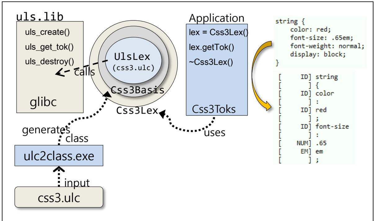
'css3.ulc' is selected to tokenize css3 file and the ulc file is processed by the program 'ulc2class' to generate the header file 'Ccss3Basis.h'. The file has token definitions for each css3 token and inherits the class 'UlsLex' in the c++ library.
