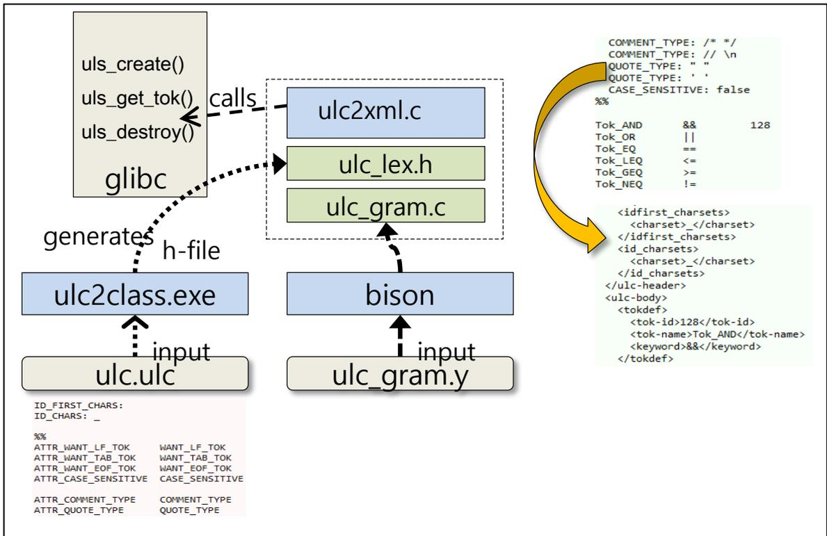
'ulc.ulg' a rough and old description of ulc file and 'ulc\_gram.y' is an yacc grammar file. The executable is a program linked with the 'uls' library. The file 'ulc.ulg' is processed by the program 'ulc2class' to generate the header file 'ulc\_lex.h'. The file has macro definitions for the token definitions.
