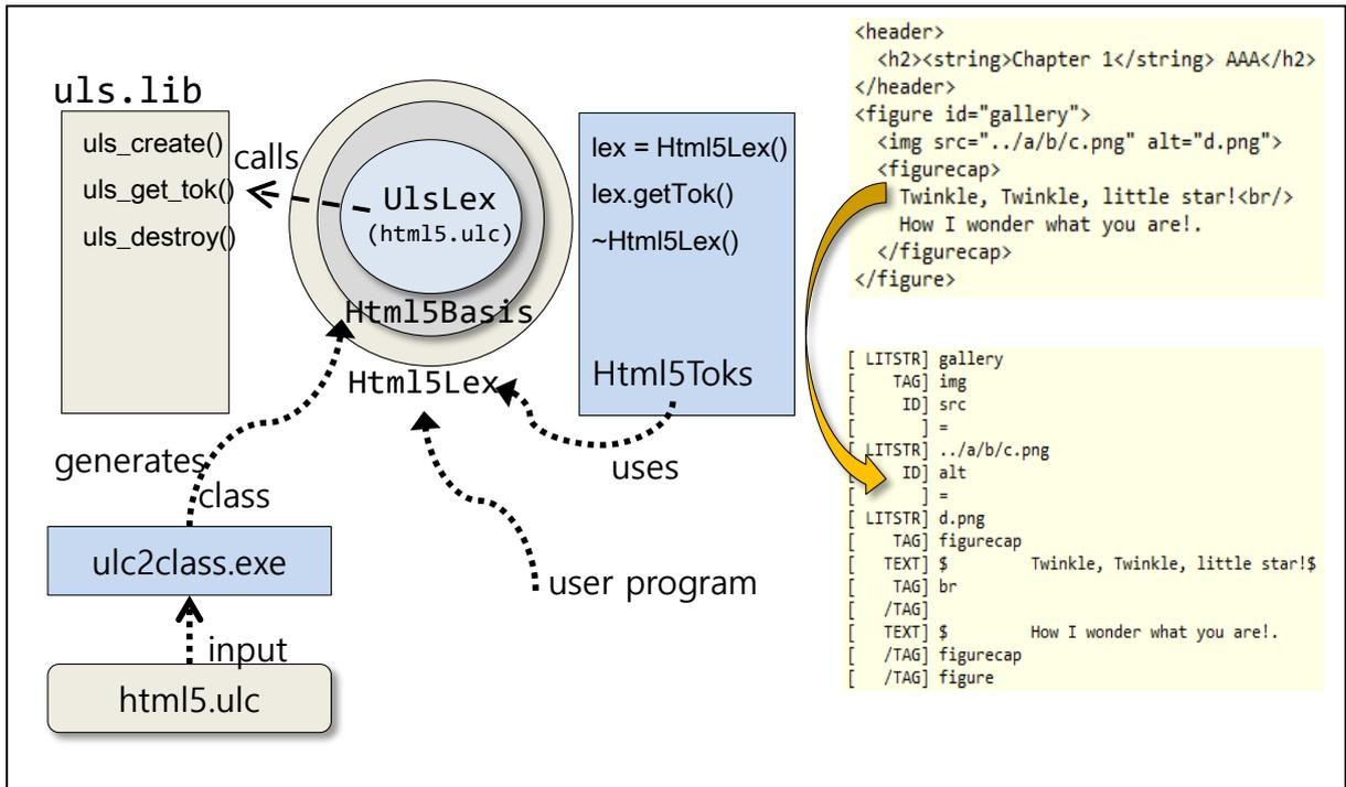
Above html5.ulc is processed by the program 'ulc2class' to generate the header file 'Html5Basis.h'. The file has token definitions for each token and inherits the class 'UlsLex' in the c++ library.
