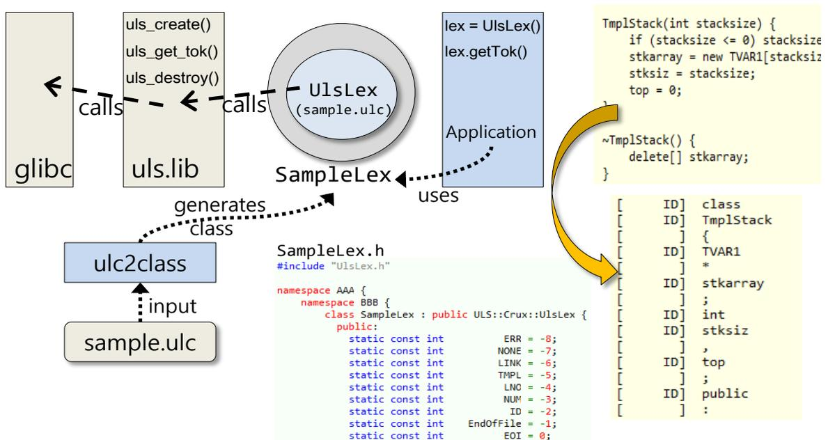
To begin with, a proper ulc file must be selected. Above sample.ulc is processed by the program 'ulc2class' to generate the header file 'SampleLex.h'. The file has token definitions for each token and inherits the class 'UlsLex' in the c++ library.
