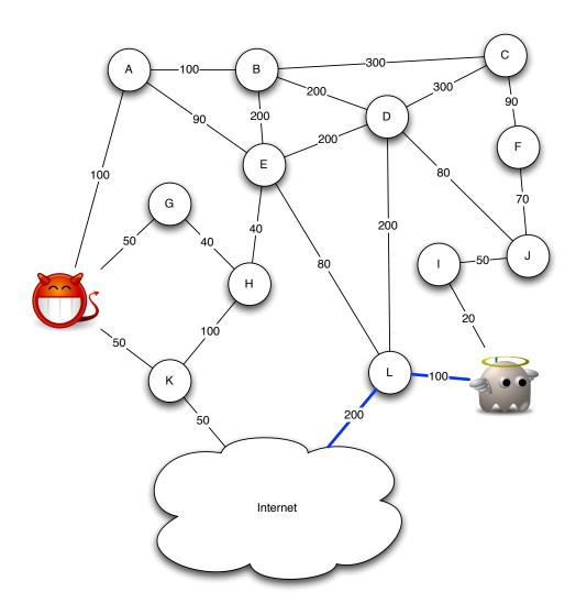
To route traffic between two nodes, the nodes always choose the shortest path according to the number of hops.<sup>1</sup> The routing is thus independent of the link capacity. An example routing from B to J would be the path B-D-J. In addition, assume that routing does not transit the "Internet" cloud in the diagram (that is, it won't go into the cloud and back out).
